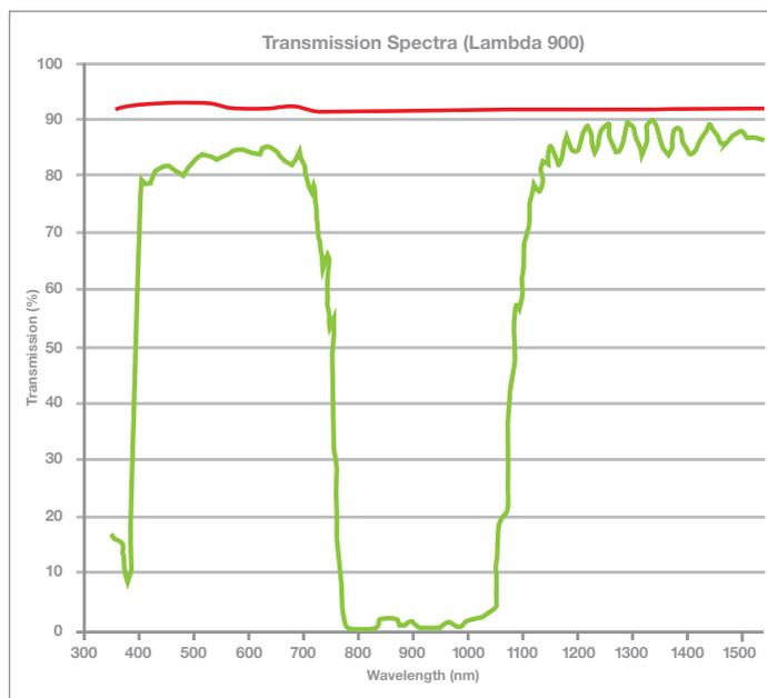
Data was taken at 5 nm sampling. The air scan and glass slide (red line) are taken to measure noise level. The green line is the transmission curve for the IR Reflecting Film.
